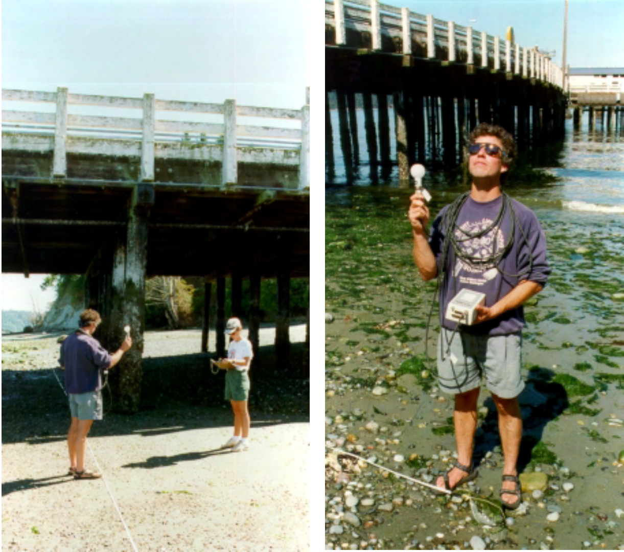
Figure 14. Photos showing our methods for recording measurements of photosynthetically active radiation (PAR) along the beach at one of the WSDOT ferry terminals, August 1998.
