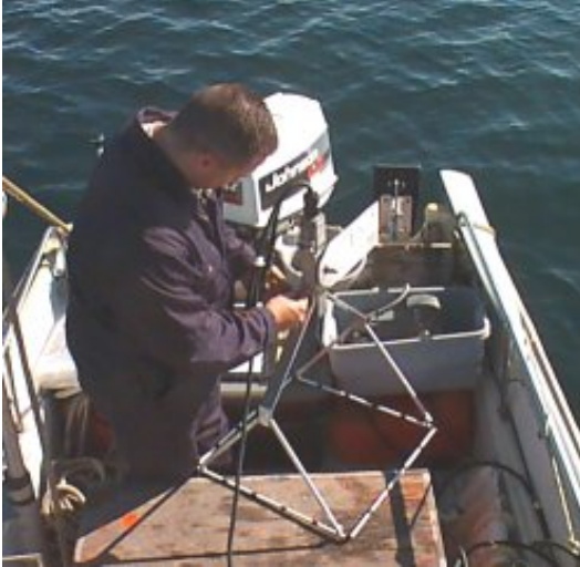
Figure 2.6. Underwater video camera showing the 0.5m x 0.5m image frame.
