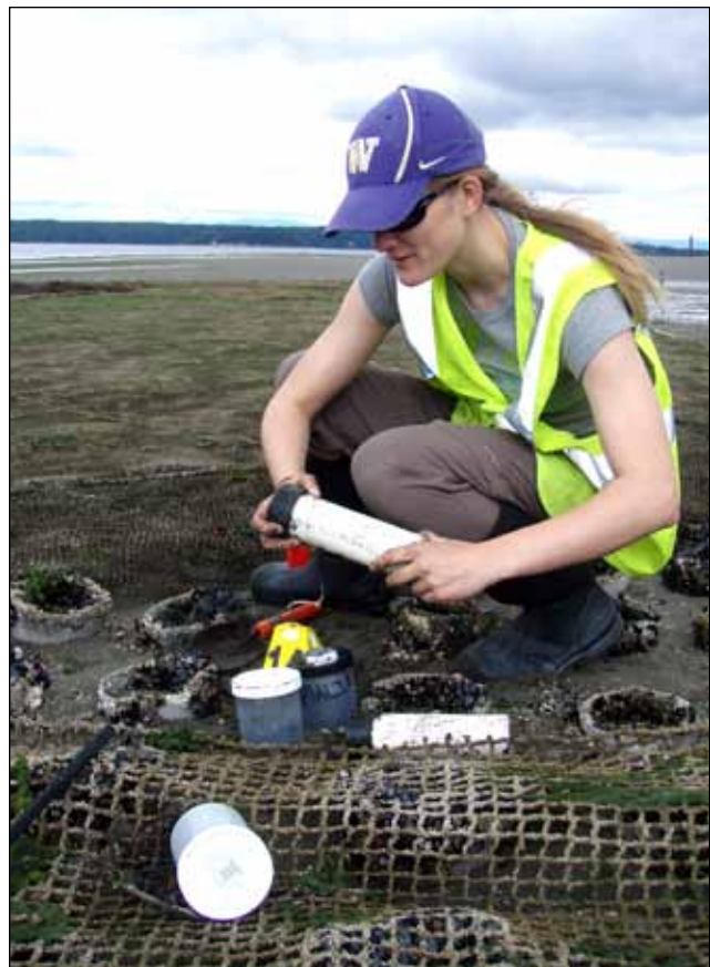
Figure 3. Technician Brittany Cummings collects core samples at a planting effects site in Case Inlet. Core samples are sieved and processed in the laboratory to investigate the effects of aquaculture gear on the community of organisms living within the beach sand (photo credit: P. Sean McDonald).
